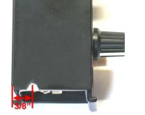
4) Tuck wires into notch and stick battery holder to side of QuikFinder using provided double sided tape.
