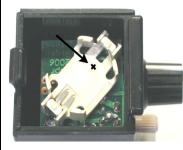
3) Press AA battery electrodes into coin cell battery holder with red wire to positive (+) contact and black wire to negative (-) contact.
