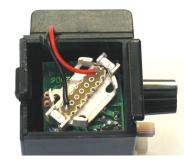
2) Place Quikfinder with knobs to right, side up as shown. 3/8<sup>th</sup> inch from back, make 1/4<sup>th</sup> inch deep notch in side using drill, clipper or other tool as shown. This will not void your warranty.
